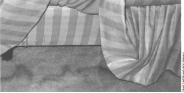
The skirt of the sofa acts as a collection device for the soot in the air caused by the gas log. Note the ring of soot deposited around the bottom of the skirt.
